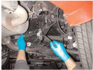
3. Gather the smaller anti-sway bar and bushings from the kit. Apply grease from one of the supplied grease packets to the inside of the bushings. Next, lay the new bar next to the factory bar and position the new bushings in the same area as the bushings on the factory bar. Transfer the factory brackets over to the new bar. Illustration 3.
