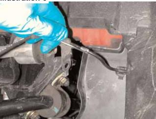
7. Using a 5mm Allen wrench and a 14mm combination wrench, remove the nuts attaching the top of the anti-sway bar end links to the anti-sway bar. Remove the end links from the anti-sway bar. Using a 14mm combination wrench, remove the nuts that secure the anti-sway bar brackets to the vehicle. Remove the brackets and the bushings from the bar. Illustration 7.
